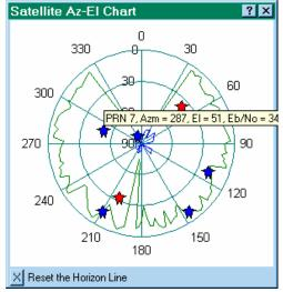
active satellite. Over time the horizon trace will fill in as satellites move through their orbits. It takes at least twelve hours to complete a horizon trace as shown above. Note that in this trace several large trees block the satellites between 150 and 190 degrees azimuth. No satellites are seen at low altitudes to the north because of their orbit inclination relative to the latitude of this station (about 39 degrees North).
