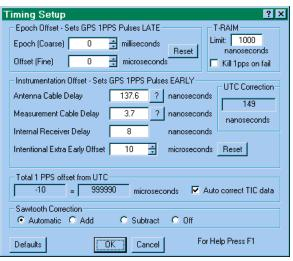
in signal propagation through the coax cables and hardware gates must be accounted for so that the leading edge of the 1pps time mark arrives at its termination at exactly the correct instant. Second, large offsets in the 1pps time mark are useful in the precise measurement of event time duration or delay.
