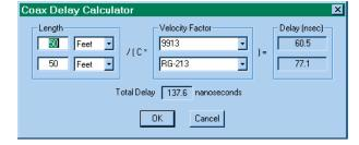
**Length:** Enter the length of each run of coax and select the units. If you only have a single run of coax, set the length of the second coax to zero (0).
