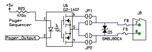
**Interface:** The interface is designed to connect directly to a variety of pager terminals by using the terminal's "Busy" line. This includes thee Zetron 2200, Kantronics Model 2000, Motorola Unipage M15 Paging Terminal and the GlenAyre GL3000.
