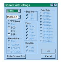
dynamically generated each time Tac32 starts and should accurately reflect the available COM ports on your computer. This includes both normal and high performance ports such as those that are part of RISC and ASIC processor boards. Ports are listed here even it they are in use by another program. If you choose a port that is already in use an error message will appear.
